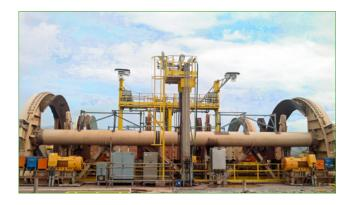
The product LaseRCD - Rail Car Dumper is a solution applied for the fully automated detection of material volumes as well as objects while the rail cars arrive at the dumping station before tipping.
