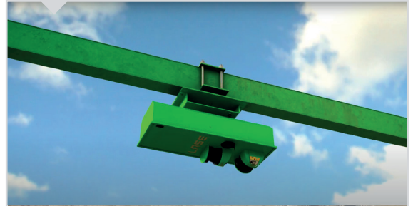
Two 2D laser scanners are positioned on a frame above the track.
