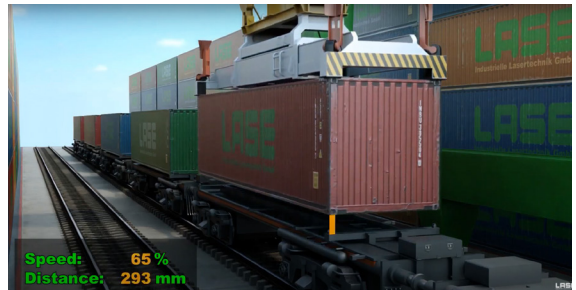
The application determines the distance to the ground and automatically reduces the speed.
