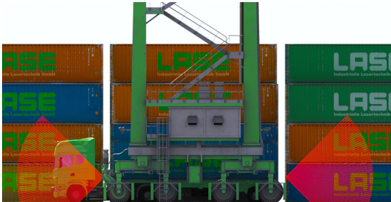
The sensors observing the area in front of the crane.
