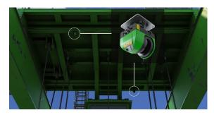
Retrofit solution: The LaseLCPS-2D sensors are mounted underneath the trolley.
