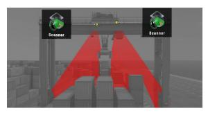
The sensors continuously measure the distances to surrounding containers to avoid collisions.
