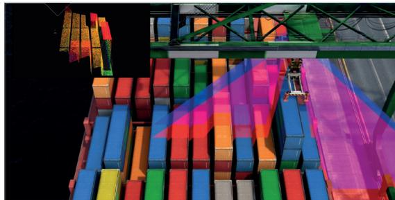
The sensors continuously monitor the working area.
