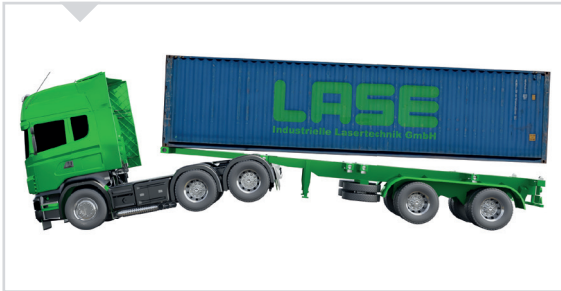
Dangerous situation: A truck trailer lifted by twistlocks.
