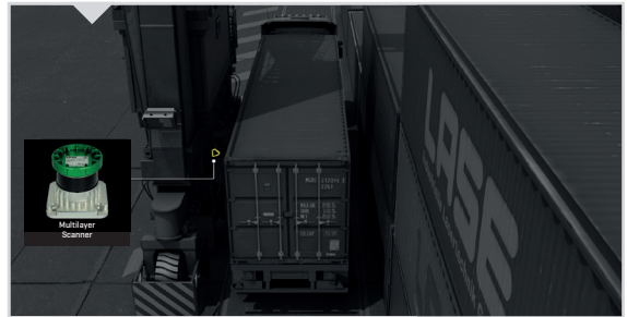
The multilayer scanner on the crane detects the separation between the chassis and the load on the truck.
