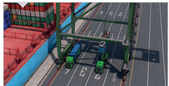
LaseTPS positions the truck optimally for un- and loading.
