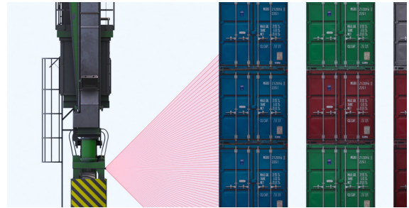
Mounting position of the laser scanner.
