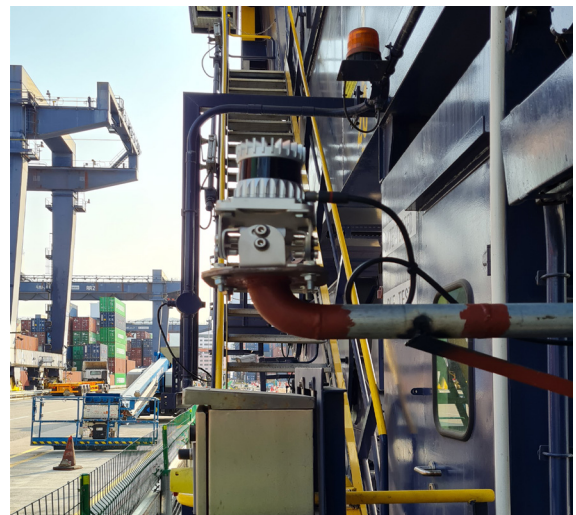
Mounting on the side of the RMG looking over the fence.
