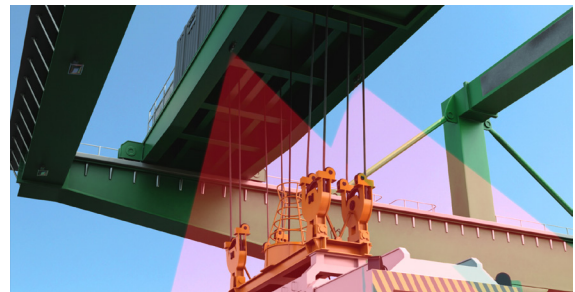
Retrofit solution: Two 3D scanners are installed under the trolley of an automatic stacking crane.
