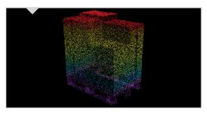
With the 3D profile created, the dimensions and volume of the cargo are determined.
