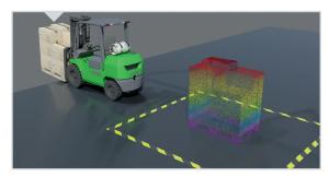
The application creates a cuboid that "encloses" the piece of cargo. These are the maximum dimensions.
