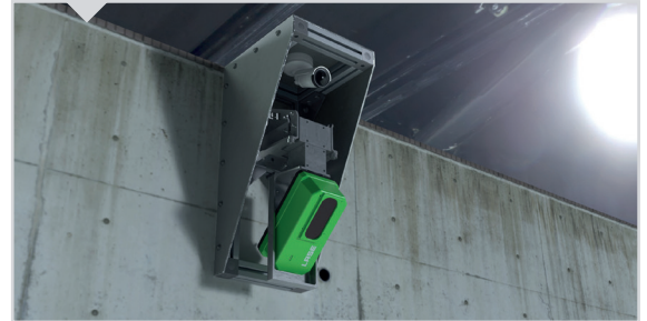
The laser scanners can be flexibly mounted on the ceiling, walls, or individual mounting constructions close to the measuring site.
